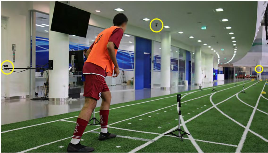
**Figure 8:** Sprint test data acquisition. Force plates (installed under the turf, dotted area) and high-speed video cameras (yellow circles) are used to acquire detailed performance data during assessment and training. Our novel motion capture system allows marker-less motion analysis, i.e. no need to attach any markers or sensors onto the player.
