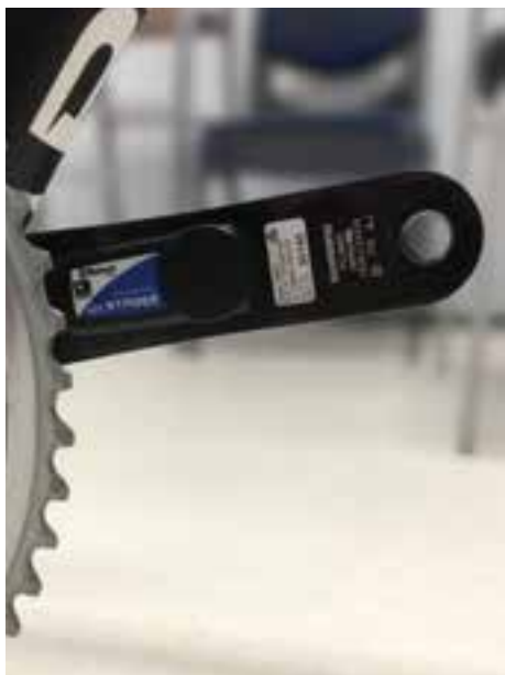
Figure 3: Crank-based power meter.
