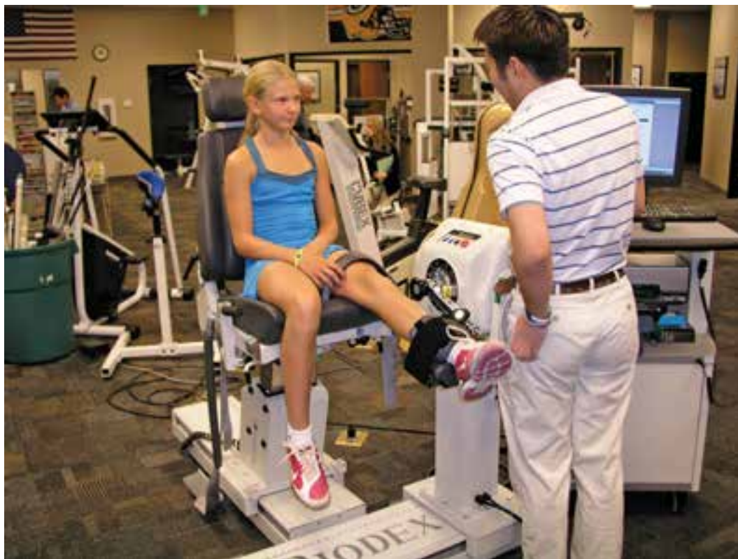
Figure 12: Biodex isokinetic dynamometer used for testing quadricep and hamstring strength.
